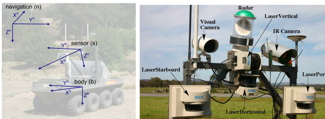
Figure 7 – Argo UGV with sensor, body and navigation frames (on the left). Variety of sensors (on the right)
